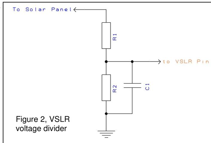
This technique allows 9V (18 cell) and 24V (72 cell) panels. C1 is used as a noise filter. A value of 0.1uF is suggested for all applications. The SSP1020 regulates the output of the solar panel by modulating the amount of energy extracted from the solar panel. Extracting a larger amount of energy will cause the voltage to go down, and vice-versa
