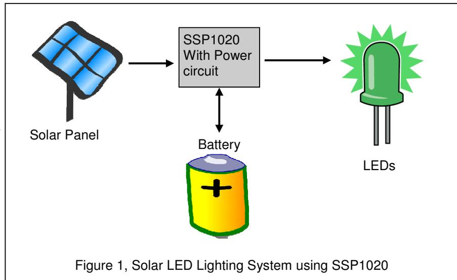
Figure 1, Solar LED Lighting System using SSP1020
